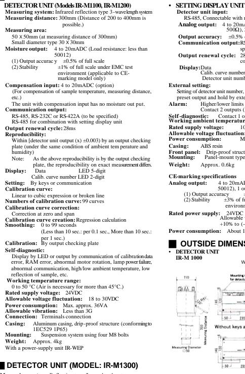
Measuring system: Reflection type 2-wavelength system **Reproducibility**: Within [detector unit output  $(x) \pm 0.015$ ] For other specifications, lease refer to Models IR - M 1100 and IR-M1200.
