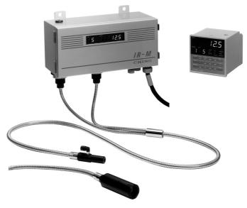
MODELS **DETECTOR UNIT** IR-M2 🔲 🔲 🔲 🔲 1: General moisture meter 2: High moisture meter Thickness meter Fiber type 0: Standard 5: Absorption type External input/output 0: Moisture output 4 to 20mADC (standard) 5: Compensation input 4 to 20mADC Compensation input Pt100 Communications interface S: RS-485 (standard) R: RS-232C A: RS-422A S for connection with setting display unit Special specification Blank: None X: Other special specifications
