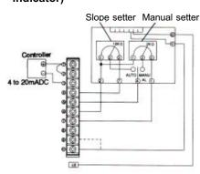
Parallel running of 3 units by current signal 4 to 20mADC
