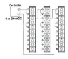
With a separate high-limit/low-limit setter
