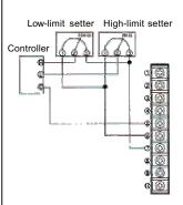
Current signal 4 to 20mADC with a setter (with output indicator)
