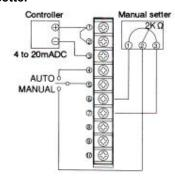
Current signal 4 to 20mADC with a separate slope setter and a separate manual setter
