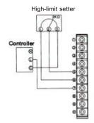
Current signal 4 to 20mADC with a separate manual setter
