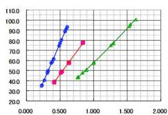
Calibration curve is a correlation between moisture determined by customer's reference instrument and IR absorption measured by IRMA.
