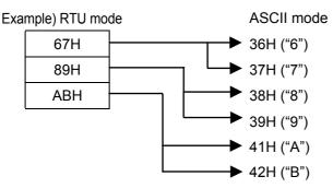
Length of the RTU-mode message is half that of an ASCII-mode message, ensuring a more efficient transmission.
