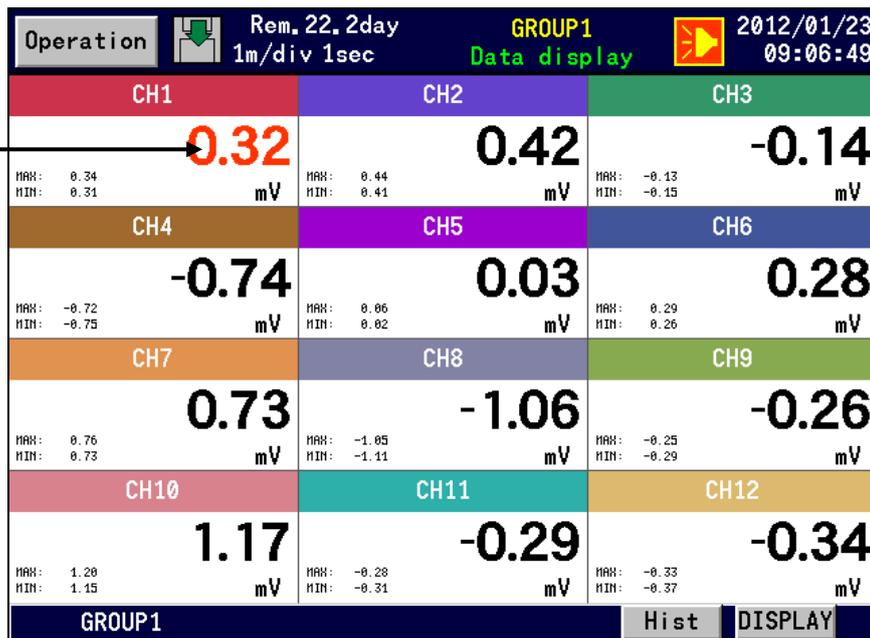
When the number of displayed channels is less than 12, maximum and minimum values of these channels can be displayed.
